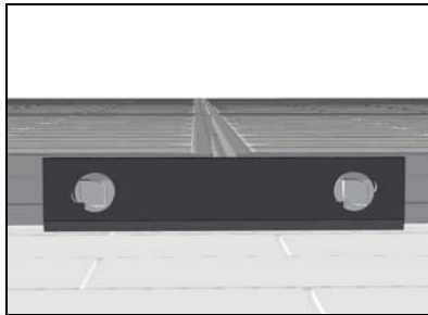
Connect PV modules
