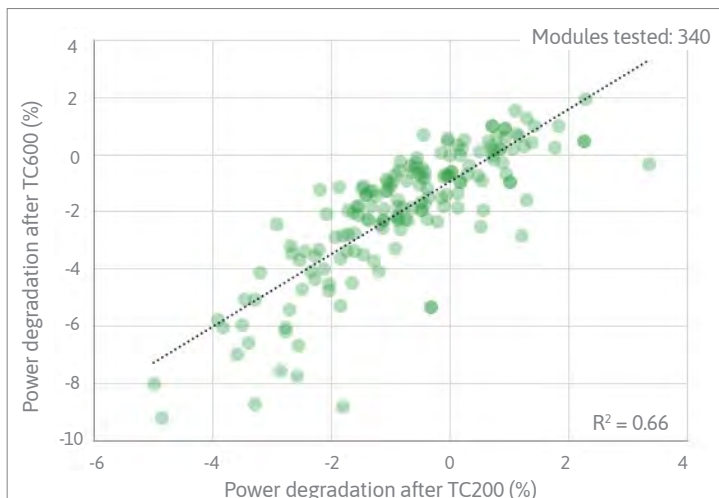
Scatterplots showing correlations between various stages of the TC and DH tests
