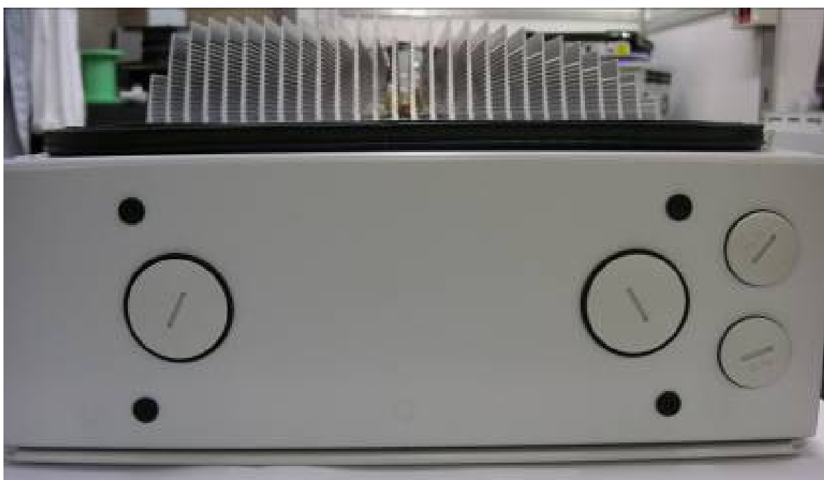
Fig. 10 - Connectors on the bottom of the inverter
