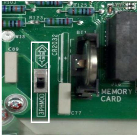
Figure 2.12 - Phase configuration 3W-Δ/ 4W- Y
