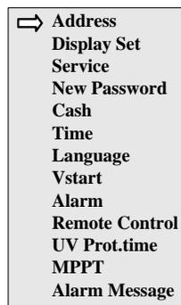
The front panel display has only two lines; therefore, the display keys must be used to scroll through the menu items and/or open the corresponding submenus (see Note 4:01). An arrow on left side of the display highlights the current selection. Once the chosen item is selected, press [ENTER] to access the desired submenu. The following section provides descriptions of each of the available submenus.
