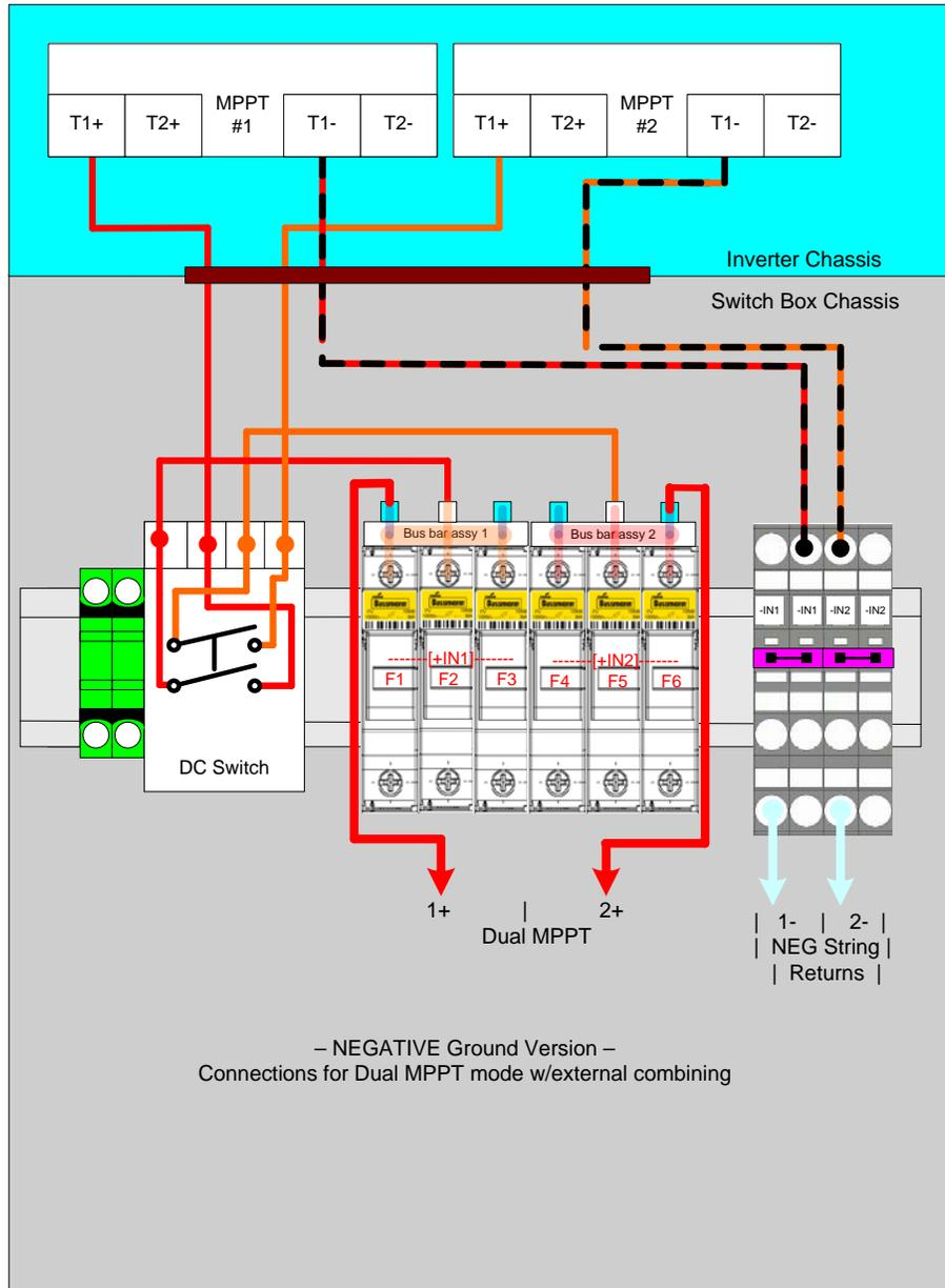
Figure 3.14c - External Combiner feed for Dual MPPT operation (Negative Ground Version)
