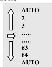
If desired, the RS485 address can be selected automatically by the system. This function is active when **AUTO** is selected from the address list.
