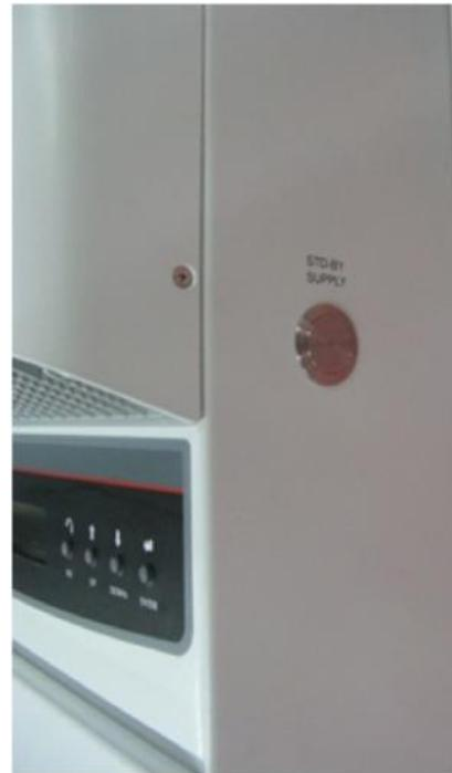
Figure 4.01- Inverter Stand-by Supply Button
