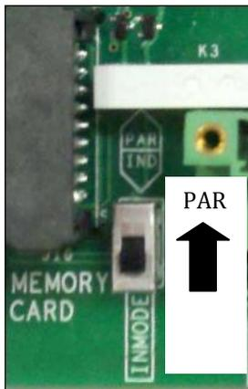
Figure 1.14a - INMODE switch set to PAR mode
