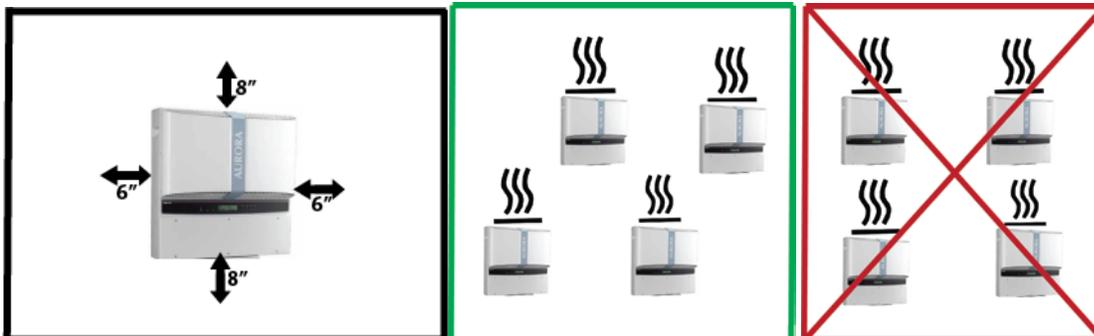
**Step 1:** Locate and mark the desired surface mounting location.
