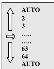
Do not select 'AUTO' as the RS485 address in a multi-unit, daisy-chain configuration.
