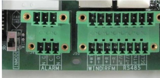
Figure 4.05 - Alarm contact terminal block
