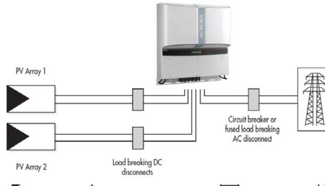
**Figure 7.02 - Simplified Diagram of a Photovoltaic System**
