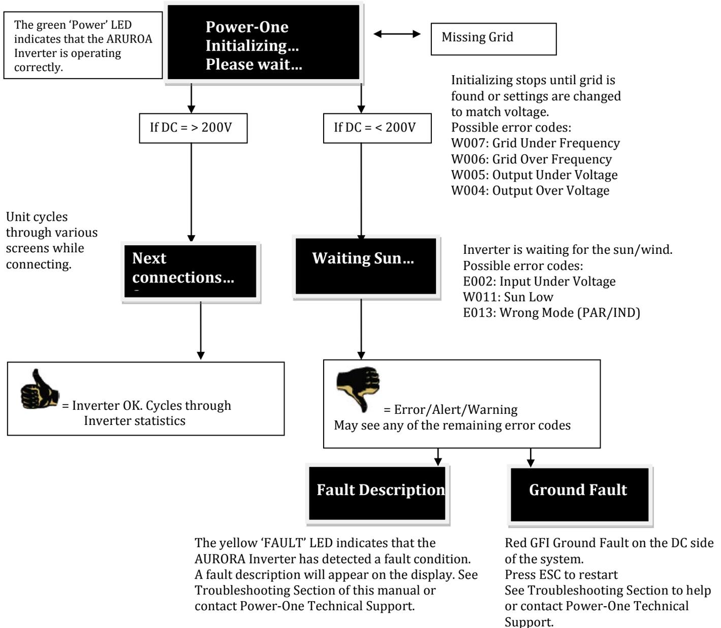
Depending on the DC input voltage present, the inverter behaves as follows:
