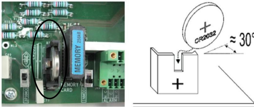
Figure 6.04 Lithium Battery Replacement
