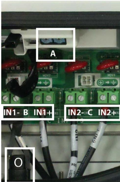
Figure 6.03 - GFD Fuse Location
