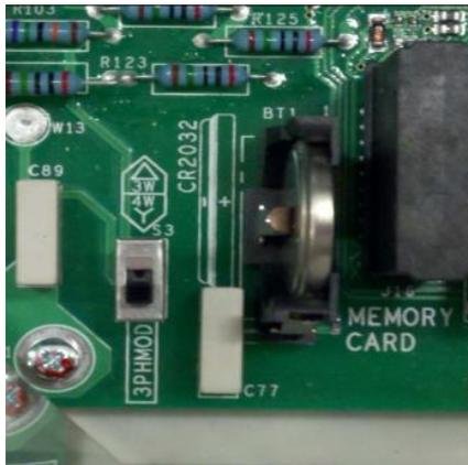
Figure 2.12 - Grid configuration; 3W- $\Delta$ / 4W-Y
