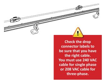
**b.** Attach the cabling to the rack using the cable clips, or you may use tie wraps.
