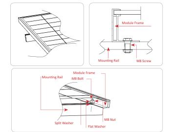
Clamp fitting: Using suitable module clamps on the LONG side of the module frame to mount the modules is "portrait orientation" mode, while on the SHORT side of the module frame is "landscape orientation" mode.
