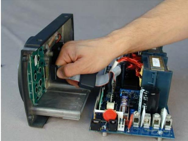
Figure 40 Reinstalling Ribbon Cable
