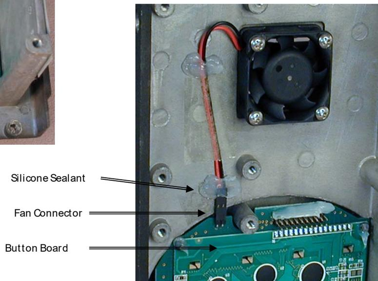
Figure 23 Disconnecting the Fan
