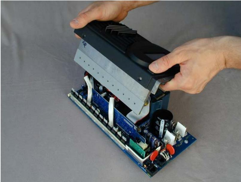
Figure 15 Heat Sink Removal
