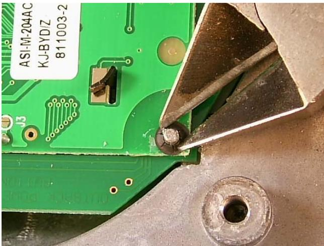
Figure 30 Inserting New Push-nut
