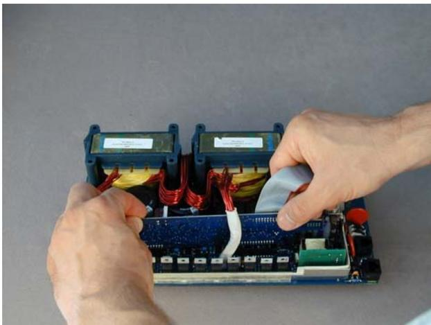
Figure 35 Inserting Control Board
