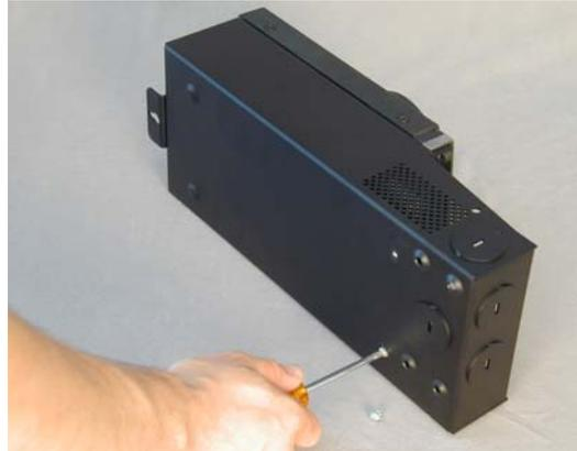
Figure 5 Back Screw Removal
