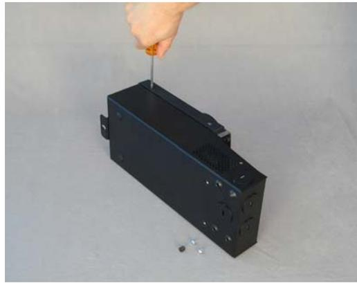
Figure 6 Side Screw Removal (part 1)
