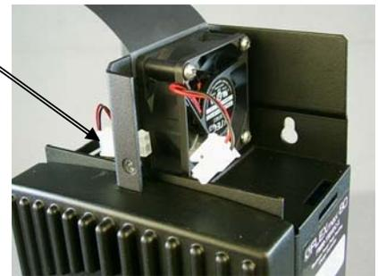
Figure 3 Removing Fan Cover
