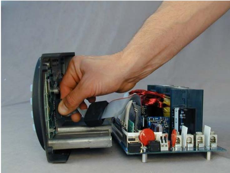
Figure 17 Cable Removal
