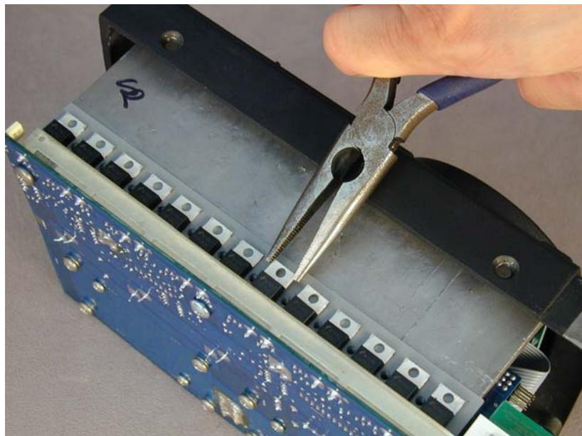
Figure 12 Freeing the FET with Pliers
