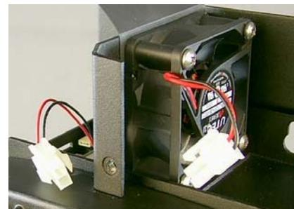
Figure 4 Removing Cable Jack
