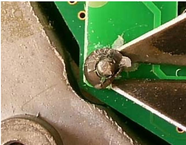
Figure 27 Removing Push-nut
