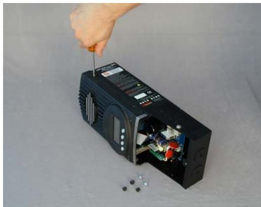
Figure 7 Side Screw Removal (part 2)
