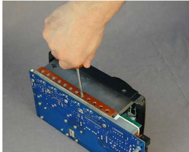
Figure 9 FET Bar Screw Removal
