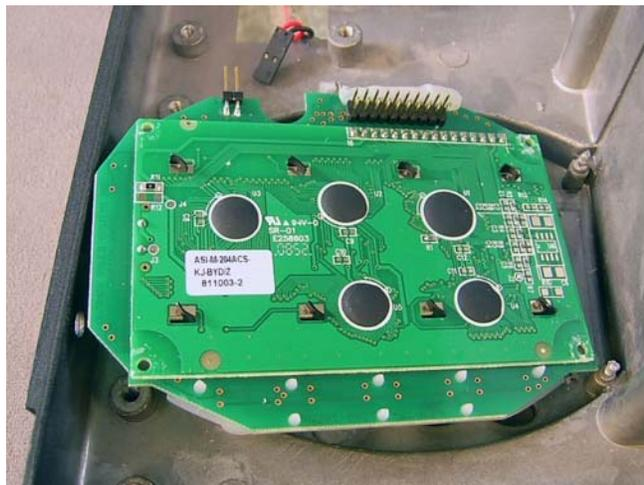
Figure 28 Removing the Button Board
