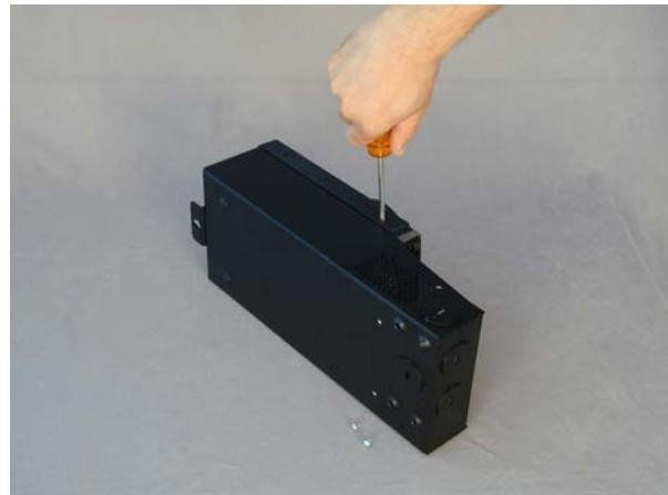
Figure 46 Replacing the Chassis Screws
