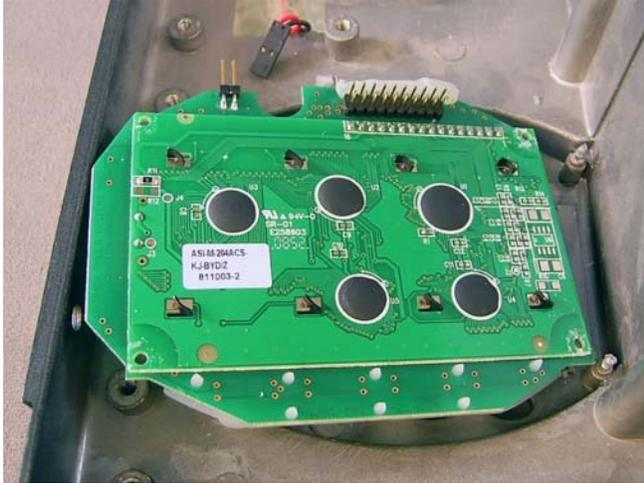
Figure 29 Inserting the New Button Board
