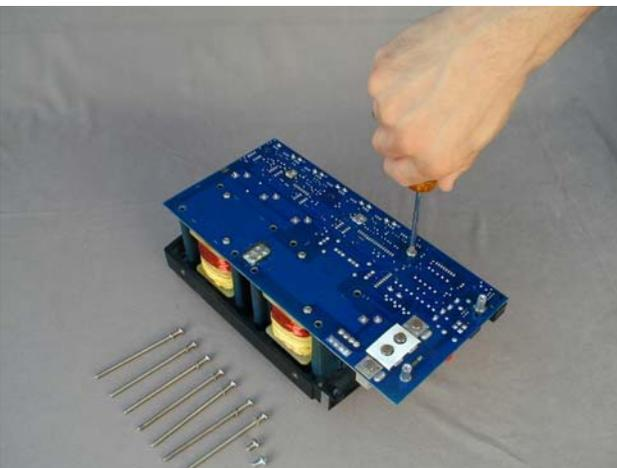
Figure 42 Installing and Tightening Screws
