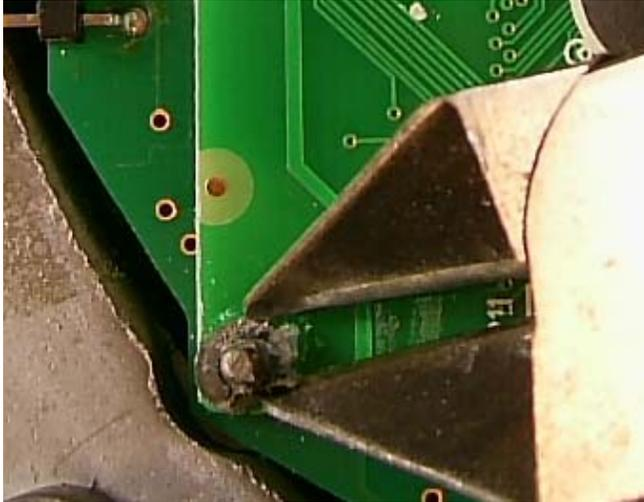
Figure 26 Deforming the Push-nut
