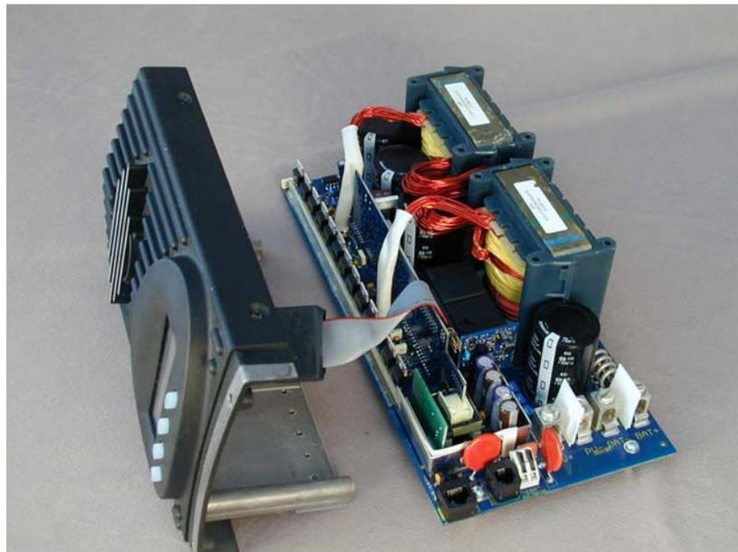
Figure 16 Heat Sink Connected to Power Board
