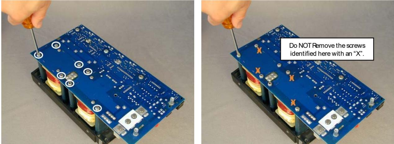
Figure 13 Bottom/Cradle Screw Removal
