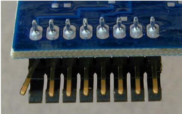
Figure 34 Bent Pin on Control Board
