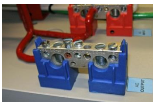
Replace the Busbar and press into place
