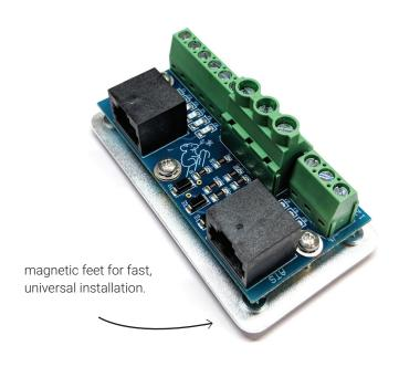
Get the most out of the Pika Energy Island's backup power capabilities with the ATS (Automatic Transfer Switch) Control Adapter Kit for whole-home backup.
