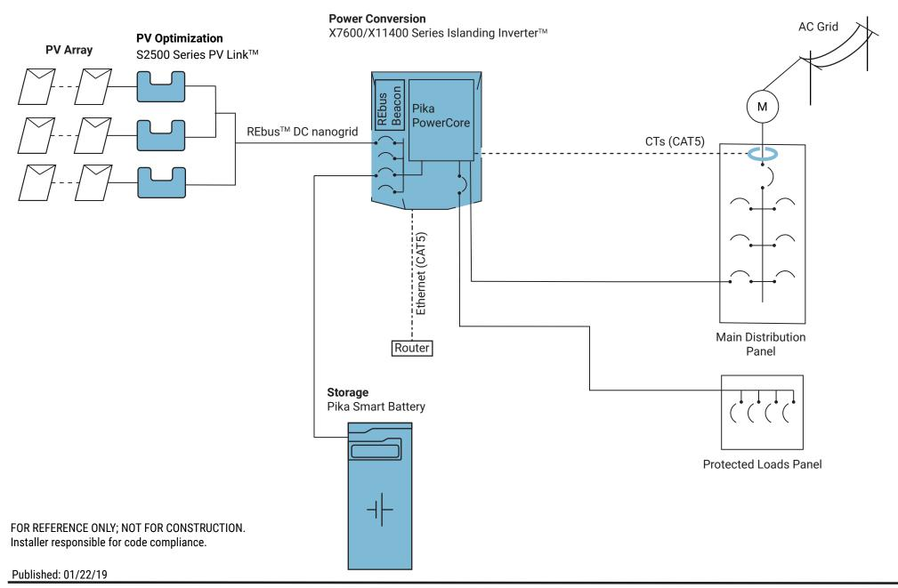
This design shows a Pika Energy Island with a Protected Loads Panel to provide backup power to loads (12 kW surge, 8 kW continuous).
