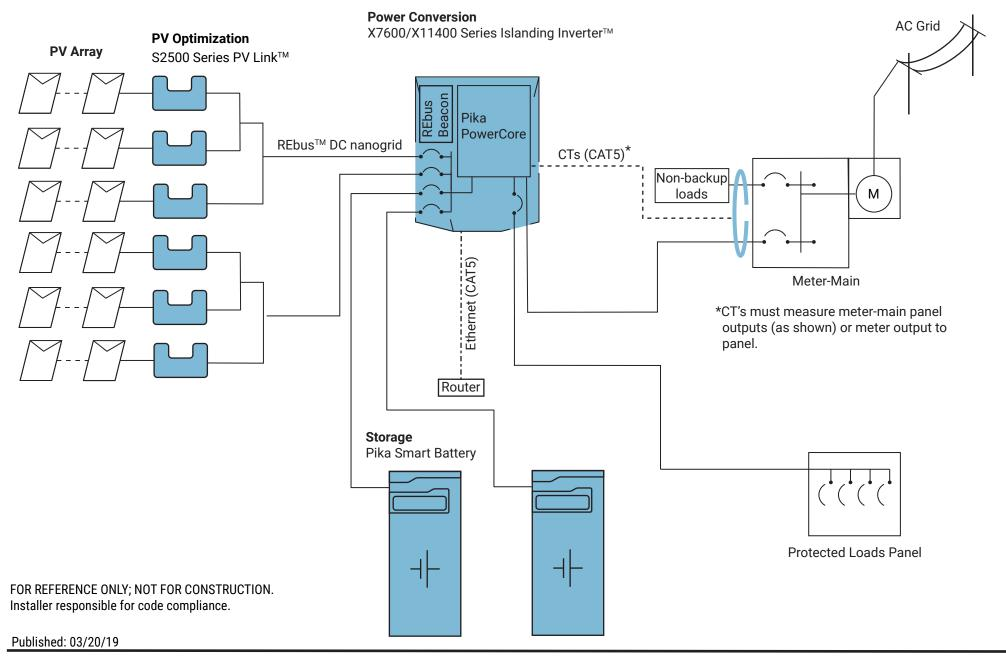
This design shows a Pika Energy Island with a Protected Loads Panel to provide backup power (12 kW surge, 8 kW continuous) connected via a meter-main. CT's shown are used to measure utility supply. They must measure all outputs of the meter-main or measure between meter and panel. This configuration is acceptable with most 200A residential services.
