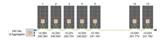
The top row of numbers is the incremental voltage rise from one microinverter to the next, and the bottom row is the cumulative line-to-line voltage overall.
