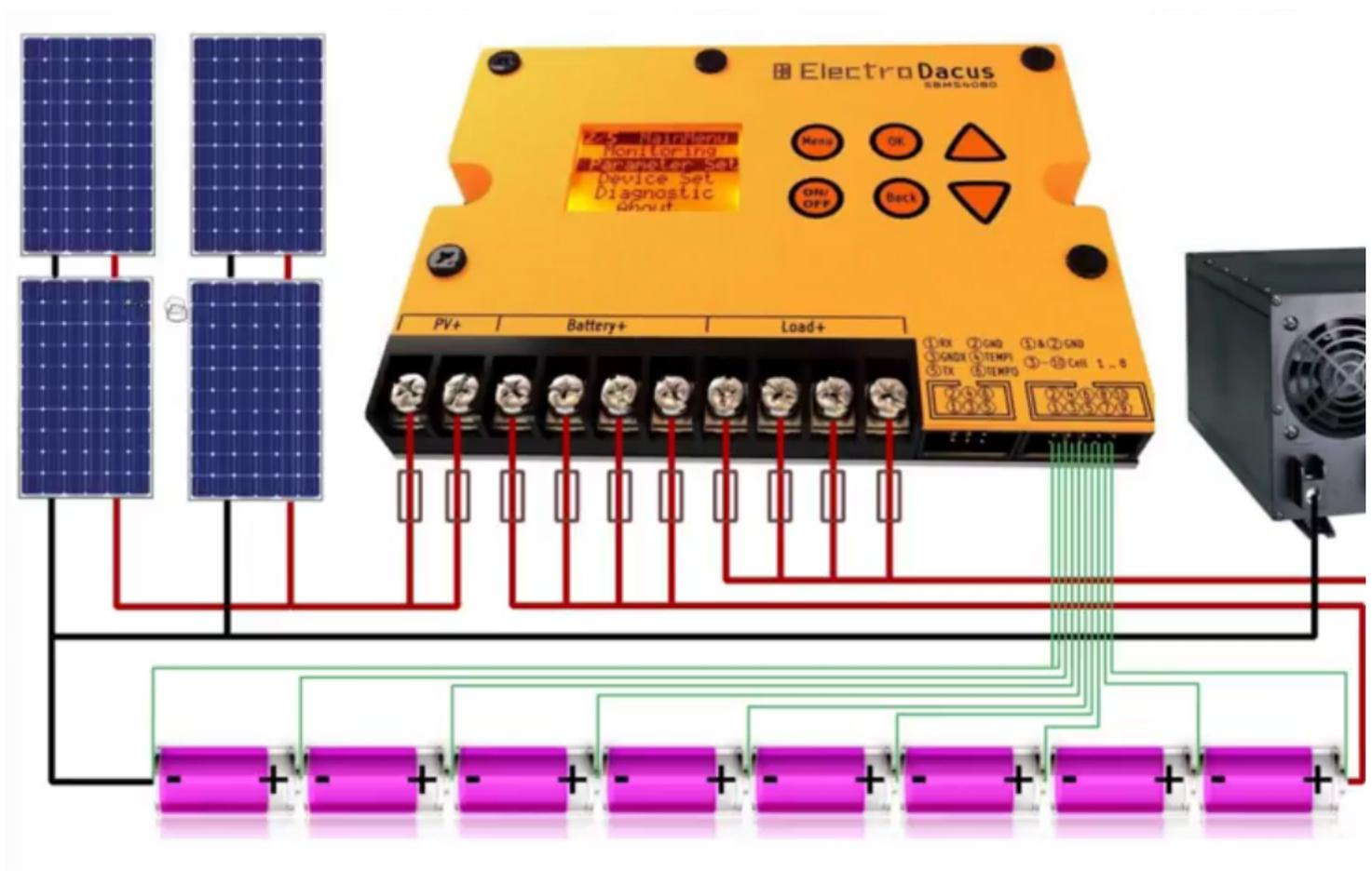
Smaller sizes as entry-configuration are also possible, but a minimum of 3 cells is required to keep the SBMS itself running.
