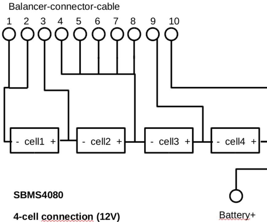
Pin No.1 and No.2 are as usual connected to battery-banks minus pol, then the first two balancer cables (from left to right) are connected to Pin No.3 and No.4, but then the other balancer cables are connected to Pin No.9 and No.10. To keep the 4 loose ends of the balancer cable from floating, they were tied up to Pin No.4 additionally.
