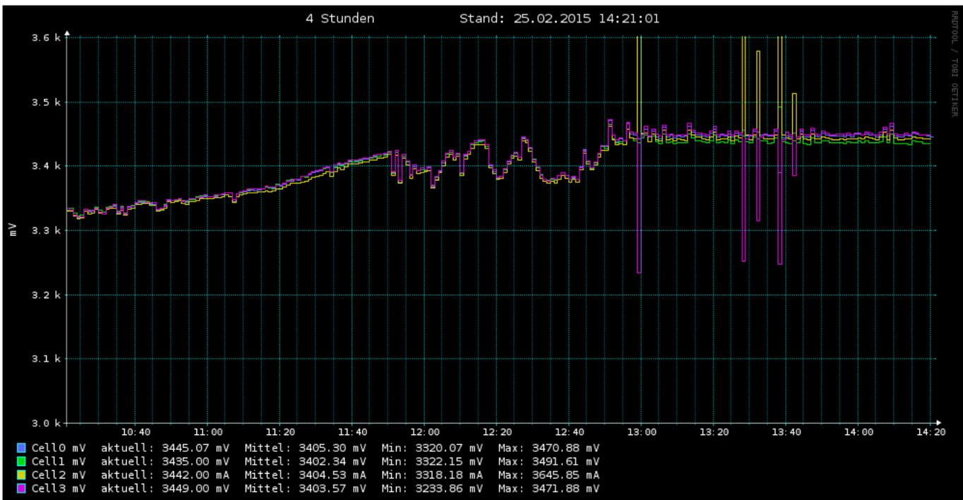
In the single-cell monitoring diagramm one can see a common voltage-level of about 3.45V with little peaks up to 3.48V. These peaks are in reality a little bit higher (like 3.5V which is the maximum per default setting), but not every peak-maximum is fully detected, due to the sampling and update frequency of 1 min. There are also a few very big peaks, which are probably artifacts caused by the switching.
