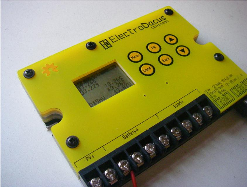
The Number 4080 means, that the Input-Amperage from Solar-panels (or other powersources) can be up to 40 Amps. The maximum output is in the range of up to 80 Amps.
