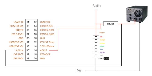
All you need for this is a 75mV current shunt. Can be 10A up to 500% and the load needs to support remote ON/OFF. (Optoisolation may be required). The current sense output from the current shunt gets connected on pins 15 and 16 on the 20pin connector.
